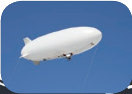
Approaches disaster-stricken sites from the sky that are otherwise difficult to reach, using a stereo camera to generate a 3D model (photo: bottom right). By quickly understanding site conditions and providing information, rescue within 72 hours from a disaster area is possible.
