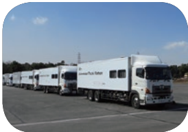
What should be seen by sensor? How should it be controlled with the collected data? The accumulation of know-how and technology resulted in platooning at a speed of 80 km per hour with an inter-vehicular distance of just four meters.
