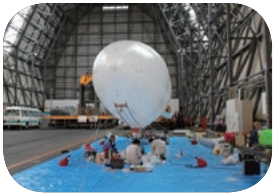
Approaches disaster-stricken sites from the sky that are otherwise difficult to reach, using a stereo camera to generate a 3D model (photo: bottom right). By quickly understanding site conditions and providing information, rescue within 72 hours from a disaster area is possible.
