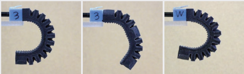
Thanks to the emergence of 3D printers, the production of robotic hands featuring a wide variety of designs has become possible. The shape of air chambers and material properties can control how these fingers bent.
