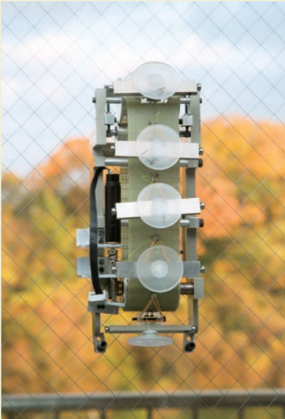
The robot is designed to climb on a vertical surface only with a well-balanced combination of caterpillars and suction cups. This robot was developed based on the design mantra that what can be done by machines should actually be done by machines.
