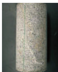
■ Granite sample on the way to fault formation. White part is a fault trace that will be a final rupture plane.
