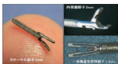
■ Micro forceps of 1mm in external diameter mounted on the tip of vascular catheter
