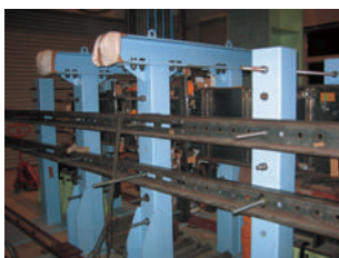
■ Experiment on the strength of a steel girder (Heavily deformed shape indicates the ductility of steel)
