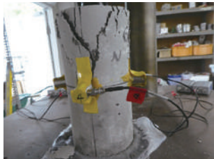
■ AE measurement to clarify fracture mechanism
