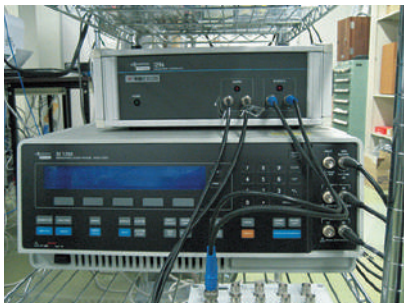
■ Impedance analyzer used in a dielectric relaxation spectroscopy method that enables dynamics measurements in wide time areas.
