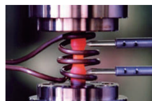
■ Multiaxial fatigue test of heat registrant alloy
