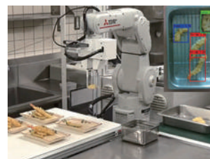
Robotic system for automatic arrangement of tempura for food serving
