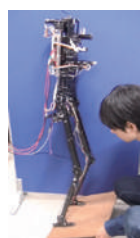
Wire-driven lightweight legged robot with high balance ability control
