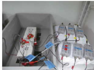
■ AE measurement to monitor rebar corrosion
