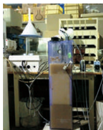
■ A lab-scale membrane bioreactor for removing persistent chemicals
