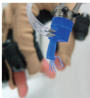
■ Remote operation by data glove of micro hand: under deployment in medical application
