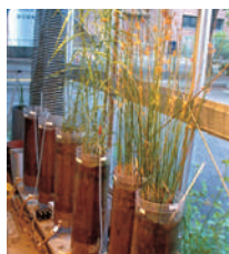
■ Landfill leachate treatment using lab-scale constructed wetlands
