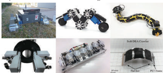
Upper left: An amphibious robot, upper middle: An in-pipe robot, upper right: A snake-like robot, lower left: A pneumatic-underdriven gripper, lower middle: A wall-climbing robot, lower right: A soft DEA-driven crawler
