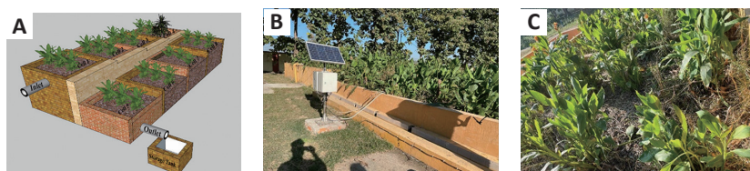
Figure 10: Diagram of HFCWs (A) and actual site photographs (B and C). Source: Singh et al. 2023b
