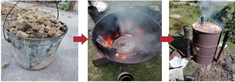
Figure 8: Preparation of biochar for constructed wetland applications. Source: Author
