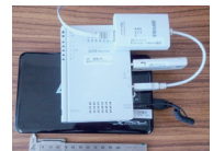
A router for satellite link (in the center of the photo) and its driving battery (a black equipment in the back of the router).
