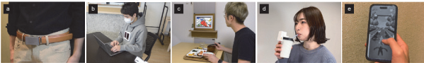
Examples of our previous research on sensor- and AI-based technologies for human behavior understanding and support. (a) belt-type wearable for daily activity monitoring, (b) self-powered sensing using energy-harvesting elements, (c) interactive visualization of eating behavior, (d) olfactory-based taste experience design, and (e) behavioral interventions for regulating smartphone use.
