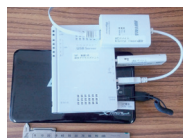
A router for satellite link (in the center of the photo) and its driving battery (a black equipment in the back of the router).
