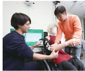
A nursing care support robot that quantitatively measures nursing care movement and teaches the correct nursing care movement
