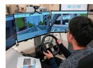
Verification of a driving support system using the drive simulator
