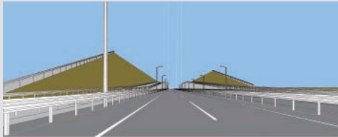
A simulation of the longitudinal gradient illusion (right) placed between the Anagawa Higashi Interchange and the Kaizuka Interchanges on Tokyo-bound Keiyo Road; Sidewalls that depict the tilted lateral stripe were placed to create the illusion. The road incline appears steeper when compared with the road side with no walls (left).
