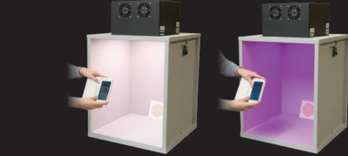
By making supplemental light of appropriate spectral distribution shine on objects, people with congenital color deficiency will be able to distinguish the color of those objects.
