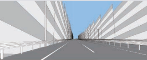
A simulation of the longitudinal gradient illusion (right) placed between the Anagawa Higashi Interchange and the Kaizuka Interchanges on Tokyo-bound Keiyo Road; Sidewalls that depict the tilted lateral stripe were placed to create the illusion. The road incline appears steeper when compared with the road side with no walls (left).
